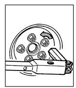
Loosen the wheel nuts – but do not remove them – using the folding wrench. (Turn the handle about 180 degrees, then flip the handle back to the starting position. This avoids taking the wrench off the lug nut for each turn.)
